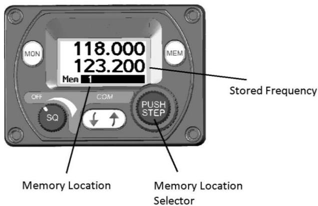
Rotating the small frequency selector knob will step through the memory locations. The standby frequency window will display the stored frequency. To store a frequency in one of the memory locations it must first be tuned and active as the primary frequency. Press MEM to enter the memory mode in the usual way. Select the channel you want to overwrite with the tuning knobs.
