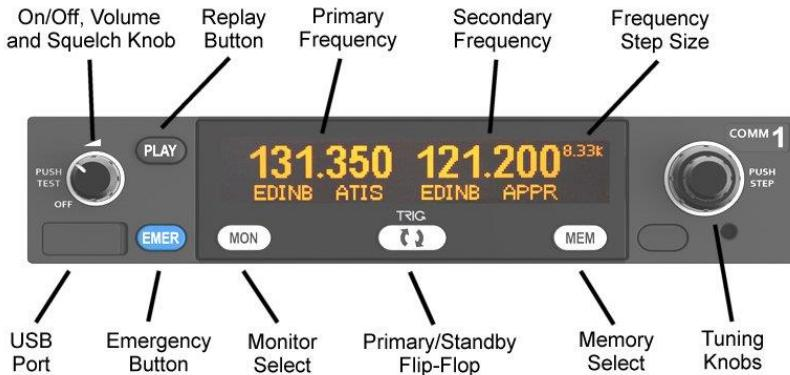
This operating manual covers both the TY96/TY97 (8.33 kHz and 25 kHz channel spacing) and the TY96A/TY97A (25 kHz only channel spacing). Any references to the TY96/97 will also apply to the TY96A/TY97A unless stated otherwise.
